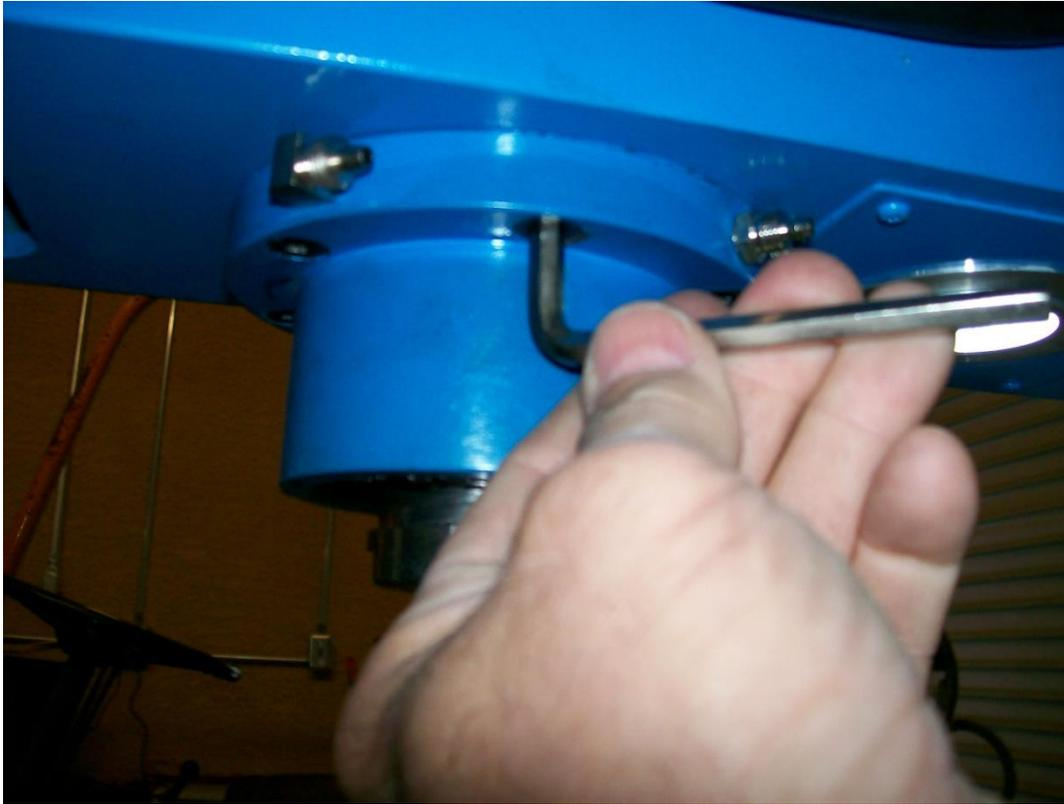
7. Place a towel on the table to protect it and tap the cartridge out from the top. Once again, paint may cause it to stick a bit, so you may need to use a hammer and a bar to drive it down from the top. CAUTION- drive against the end of the spindle NOT the pulley, as the pulley has a magnet imbedded in it for the spindle sensor.
