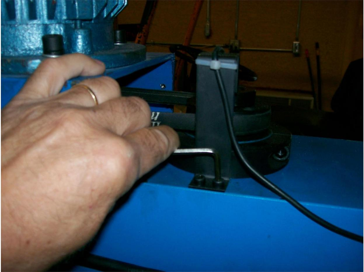
3. Loosen the 4 bolts holding the motor mounting bracket so it can slide in the slotted holes. Slide the motor and bracket enough to remove the belt from the spindle pulley. NOTE: The bracket may need a tap with a mallet to break it loose as the paint tends to stick the parts together.
