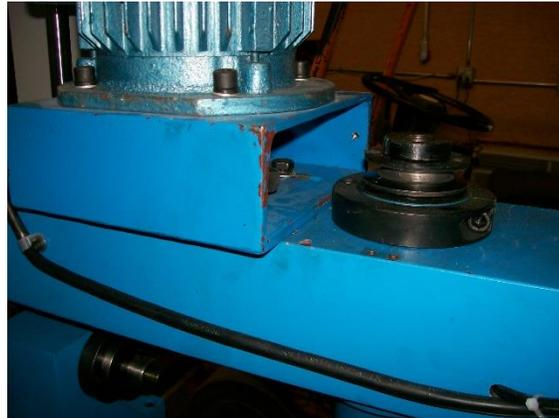
4. Remove the air coolant lines from the spindle cartridge.
