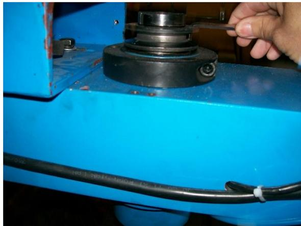
6. From below, remove the 6 bolts holding the cartridge to the mill head.
