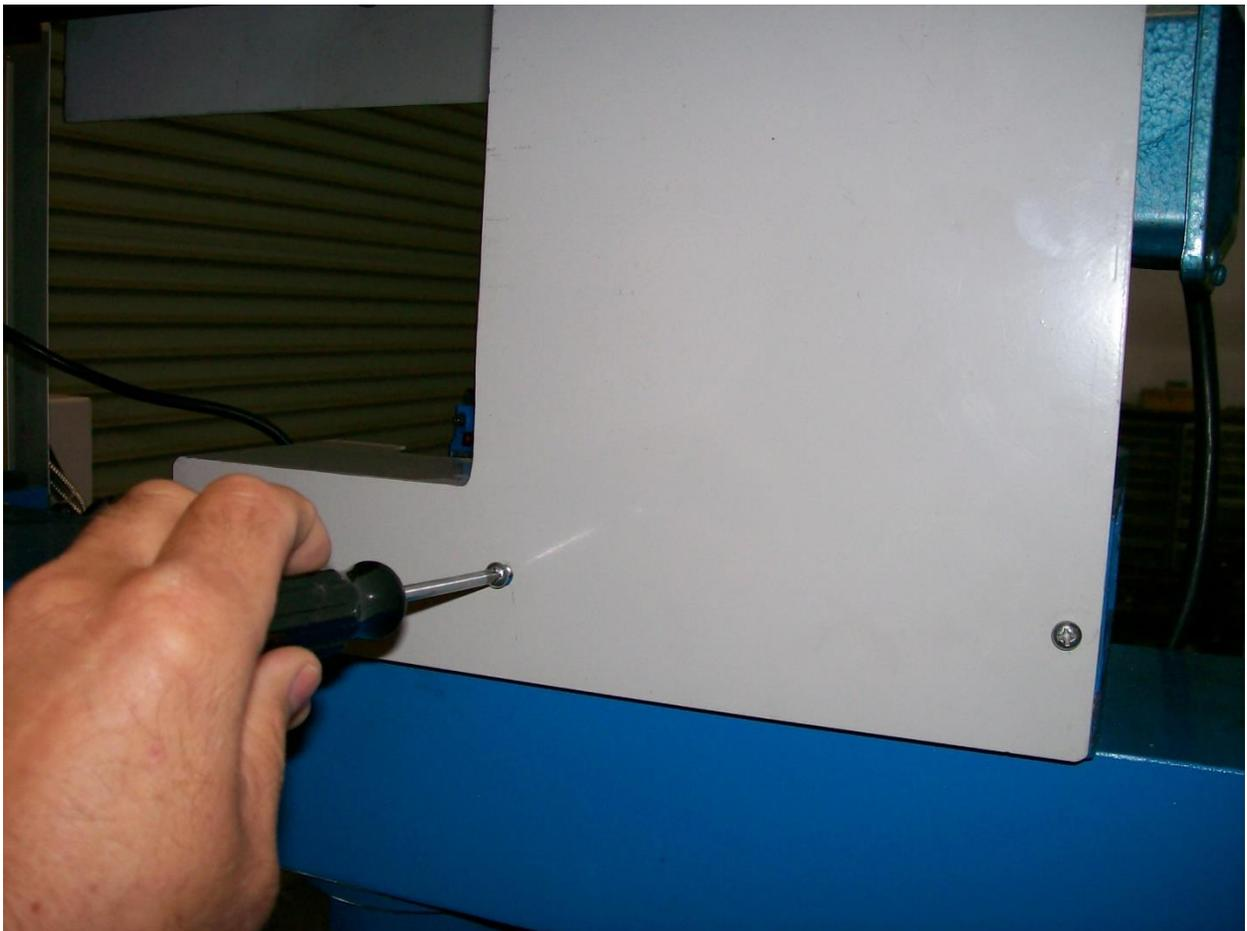
2. Move the mill head back up to about its midway point, and from the back side remove the 2 bolts holding the spindle sensor in place.
