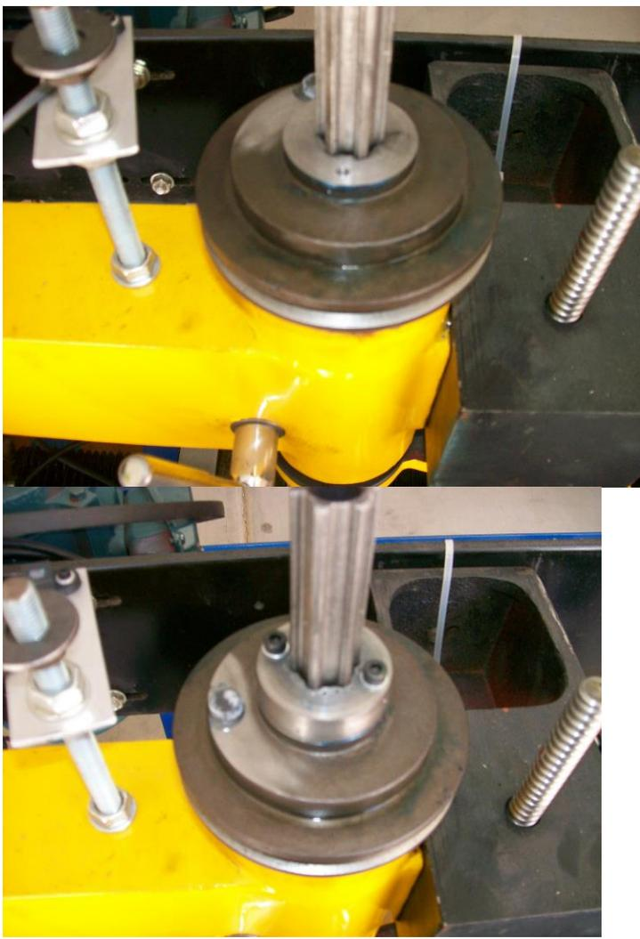
**Because the holes in the upper half of the pulley are oversized, the pulley could eventually slip due to vibration and cutting loads. Therefore you need to secure the two halves together permanently. Remove the pulley from the machine and drill two 4.5 MM holes through the remaining 2 punch marks. Tap these 2 holes with a 5 MM X 0.8 tap and place 2 more 5 MM bolts into them. Because these holes are tapped together and not oversized, the 2 pulley halves cannot slip out of place.**
