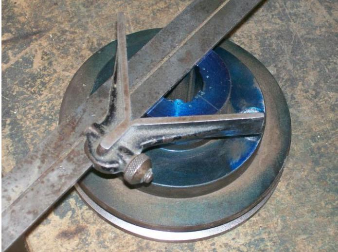
**Now select 2 opposite holes and drill them all the way through with a 4.5 MM drill. Measure the depth of the splined portion of the pulley , chuck it in your lathe and set your parting tool blade so that it cuts the pulley as close to 50-50 as possible. Go slowly and use lubricant, as you will cut through the drilled holes as well as the splines.**
