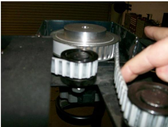
6. Once your belt is back in place, remove your support piece and run the mill head down a bit then back up and measure the distance again to see if you got it right. That covers the main adjustment.
