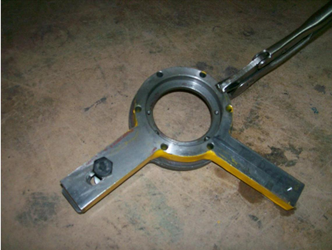
4. **Clamp the assembly in your vise and using a 6mm drill, go through the 6 original holes in the bracket just enough to create a dimple in the stiffener plate.**
