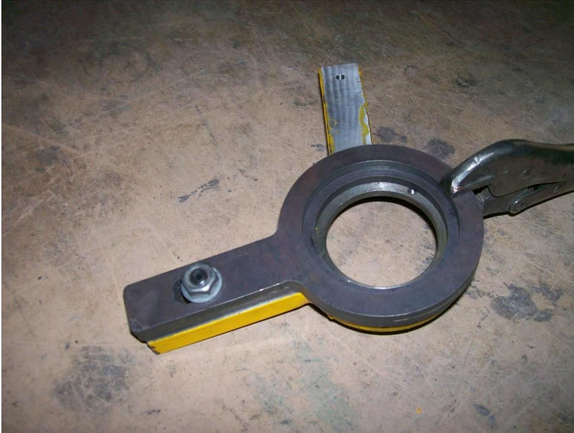
3. Once the assembly is aligned, tighten the bolt in the ball screw hole and add a vise grip to the other end to keep every thing aligned.
